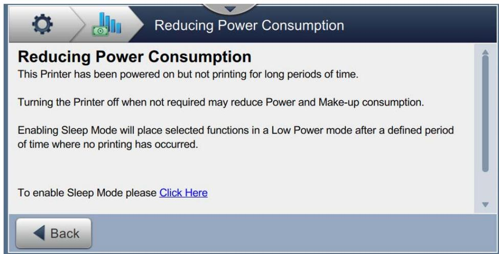
Figure 2-6: Reducing Power Consumption Screen
